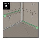
Place the support in position, aligning the top edge of the support piece with the lower of the two marked lines.
