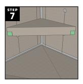
Smooth out any excess joint sealant on the underside of the supports with a corner putty knife. Dry-fit the bench in position to ensure it sits evenly and level on the supports.
