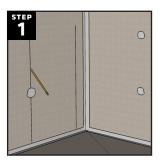
Decide on a suitable corner in your shower for your shower bench to be installed, ensuring it will not interfere with a proper standing position based on your shower head placement. Mark the positions of the two studs which are closest to the corner on both walls (e.g. a corner stud and another stud 16" OC from the corner stud).
