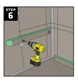
Attach the support to the wall using a HYDRO-BLOK washer and included 3 ½" screw at each stud location. Repeat steps 4 to 6 for the other side support, applying additional joint sealant to the face where the supports will meet in the corner.
