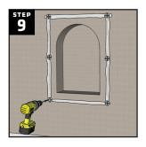
Install HYDRO-BLOK washers and screws at the corners and along the vertical seams every 12" so that the washer covers half of the niche and half of the wallboard. For double wide niches, place washers and screws at the top and bottom of the centre stud as well along the horizontal seam.
