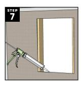
Apply a ½" continuous bead of HYDRO-BLOK joint sealant on all 4 inner edges of the wallboard in the opening.
