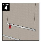
Using a utility knife, cut the horizontal lines first, using those cuts to ensure that the vertical cuts will be located in the middle of a wall stud on each side.
