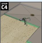
To install the straight extension piece(s) apply a ½" continuous bead of HYDRO-BLOK joint sealant along the shower pan notch, along the exposed foam edge of the shower pan, and along the corner extension notch. Apply a generous amount of joint sealant to the wallboard where the ends of the extenstion(s) will be located.
