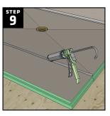
Apply an additional ½" continuous bead of HYDRO-BLOK joint sealant over the seam between the shower pan and the extension and use a putty knife to smooth out the sealant.
