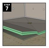
Place the extension into position by slowly angling it into the joint sealant and then lowering it into the thinset. This will ensure good adhesion of the joint sealant with the foam without forcing the thinset up into the joint.
