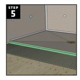
Using the same thinset material used in the shower installation (you may have to re-mix or make a new batch if the thinset is too hard from using it for the shower pan installation), apply thinset on the subfloor where your extension will fit. Ensure the trowel lines travel away from the shower pan. DO NOT cross-channel trowel lines or air cannot escape. Apply thinset to the back side of your extension using the flat side of a trowel.
